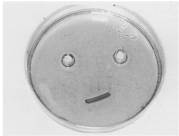
Figure 5 Results of the agar overlay test (series 4) for zinc phosphate cement, 1 h, 0% relative humidity: a zone of decoloration around each of the two test samples indicates an area of damaged cells (strip = control); the distinction between damaged and undamaged cells is sufficient.
